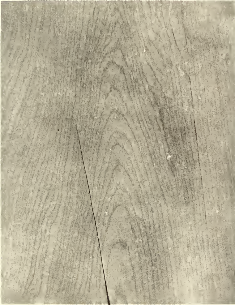
FIGURE 2-92 — Natural spiral grain as indicated by split which is not parallel with alignment of apexes of annual rings due to diagonal grain. Compare with figure 2-91.
